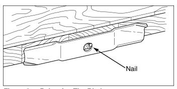
Figure 8. Balancing The Blade
